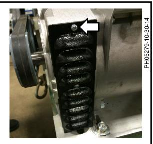
5. Put the generator in place on the two front 7/16" bolts using lock washers and hex nuts. Do not tighten hex nuts at this time.
