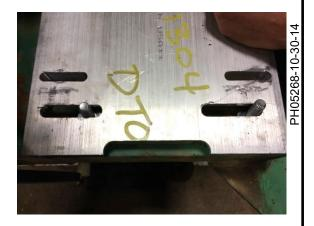
2. Position adapter plate approximately 3/4" from the edge of the chassis, on the side nearest the tire.
