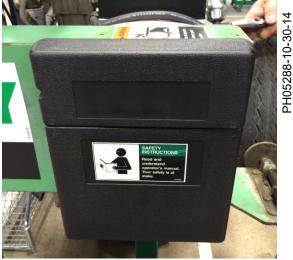
15. Attach belt guard onto the backing plate and bolt it back to the chassis using 3/8-1 1/4 screws, lock washers, flat washers, and nuts.
