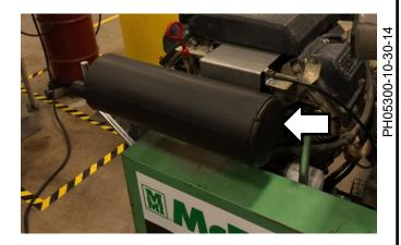
17. Install the new muffler guard and mounting hardware using  $^3/_8$ -1 screws, lock washers, flat washers, and hex nuts.
