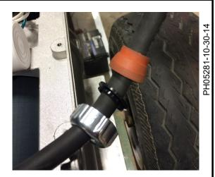
9. Push wire through 90° elbow until 1/2" of black insulation is showing and reinstall retaining nut, washer and rubber stopper.
