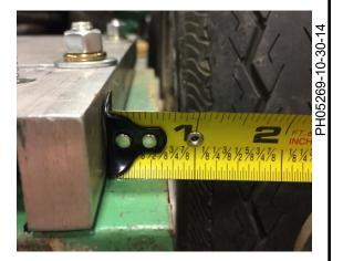
3. Bolt down adapter plate using 3/8" – 2 1/4" bolts with washers and lock washers. Note the position of the 4 mounting bolts to the outside of the plate slots.
