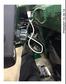
7. Remove generator cover using 5/16" nut driver.
