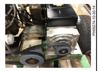
9. Position a pry bar against the generator and pull to apply tension on belts.
